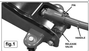
as shown in fig.2 and open the valve by turning the handle anti-clockwise, place the handle back into the jacking socket and pump for 30 to 40 seconds. When complete, close the release valve by turning the valve nut clockwise.
