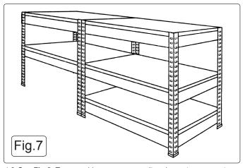
4.9 See Fig.8. To assemble as a corner unit make up two separate frames following steps 4.1 to 4.3 but with different shelving positions. Make up one frame with 3 shelves and one frame with two shelves as shown below. Ensure that the middle and top shelves on both frames are at the same height. Fix the frames together with the four nuts and bolts supplied. Place the 5 MDF shelves into position in the frames.
