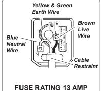
indicated in diagram. **DO NOT** connect either wire to the earth terminal.
