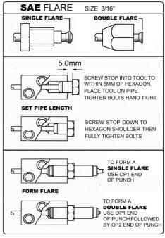
Note: A spot of grease on the end of the punch helps the flare process.
