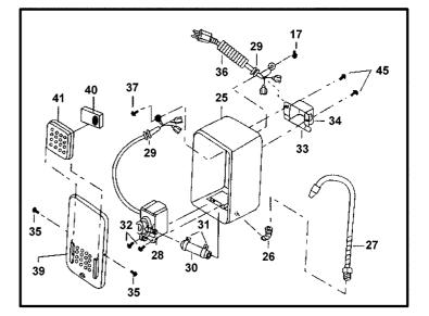
Exploded view of the pump assembly
