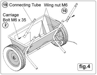
4.4 Referring to fig.4, assemble a connecting tube (19) to each leg using an M6 x 35mm hex headed bolt (2) and an M6 Wing nut (10). Firmly tighten each nut as shown in fig.5.
