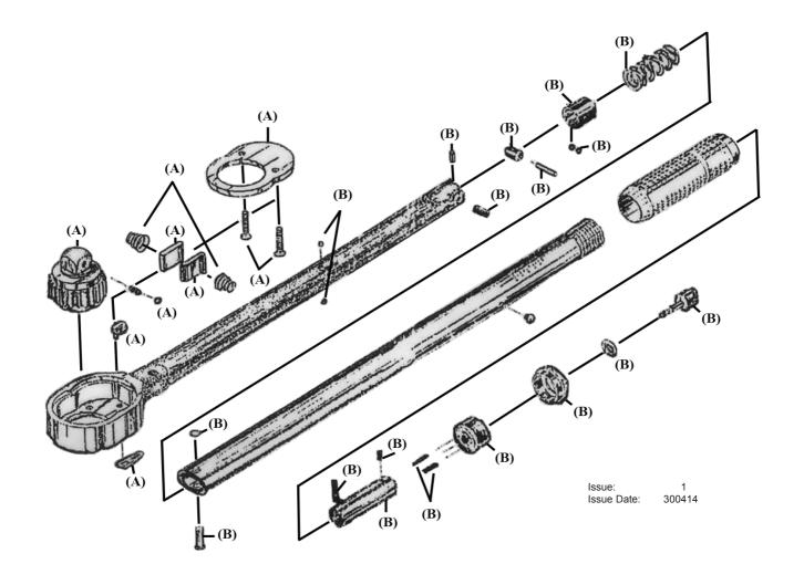
**DESCRIPTION ITEM PART NO** STW103.RK REPAIR KIT В STW103.RB REPAIR BAG
