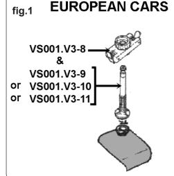
VS001.V3-9 = Ø50mm VS001.V3-10 = Ø35mm VS001.V3-11 = Ø27mm
