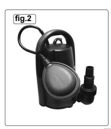
3.5. USING AS A PUDDLE PUMP: In order to draw water from a shallow depth, the float switch needs to be immobiled as in fig.3. In this mode the pump will not function automatically so, consequently, must be not be left unattended owing to the risk of overheating. The normal medium for cooling the pump motor is the water in which it is submerged, therefore excessive use in the open air carries the risk of damage.
